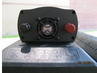
Illustration 19: Inverter prior to installation of the looped-end battery cables.
