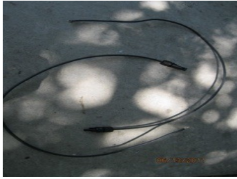
Illustration 3: Solar panel connector and open wire.
