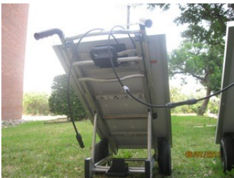
Illustration 6: Bridged panels with an open NEGATIVE (-) connector.
