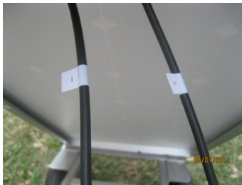
Illustration 2: NEGATIVE (-) is on the LEFT. POSITIVE (+) is on the RIGHT.
