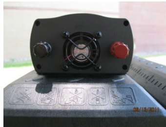
Illustration 17: Inverter prior to installation of the looped-end battery cables.
