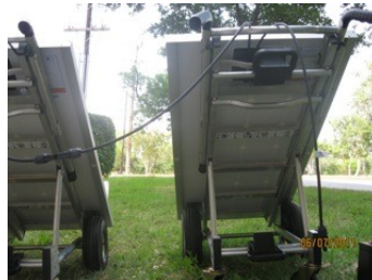
Illustration 7: Note that the POSITIVE (+) connector of the LEFT panel is BRIDGED with the NEGATIVE (-) connector of the RIGHT panel.
