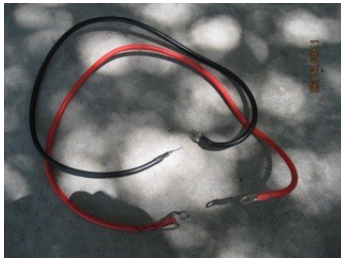
Illustration 15: Looped- end battery cables. Note that the POSITIVE (+) and the NEGATIVE (-) are not connected to each other.
