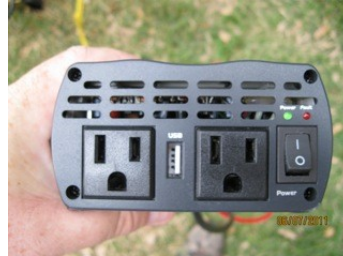
Illustration 19: Power switch and LED indicator are shown. Note that there is also a USB connector.
