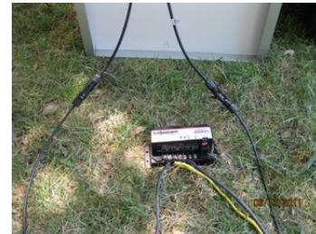
Illustration 8: (NEGATIVE (-) is on the LEFT. POSITIVE (+) is on the RIGHT)
