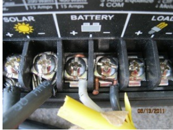
Illustration 14: POSITIVE (+) is on the LEFT. NEGATIVE (-) is on the RIGHT.
