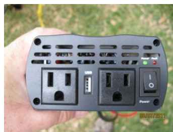
Illustration 21: Power switch and LED indicator are shown. Note that there is also a USB connector.
