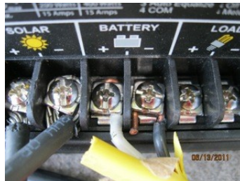
Illustration 12: POSITIVE (+) is on the LEFT. NEGATIVE (-) is on the RIGHT.
