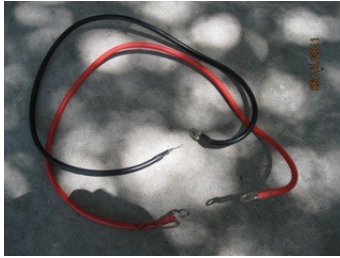
Illustration 13: Looped-end battery cables. Note that the POSITIVE (+) and the NEGATIVE (-) are not connected to each other.
