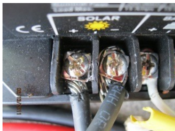
Illustration 4: BOTH NEGATIVE (-) and POSITIVE (+) are shown connected.
