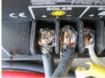
Illustration 9: BOTH NEGATIVE (-) and POSITIVE (+) are shown connected.
