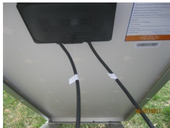
Illustration 2: (NEGATIVE (-) is on the LEFT. POSITIVE (+) is on the RIGHT)
