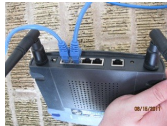
Illustration 7: Linksys Wireless G Router. Note that the the serial ports labeled 1-4 are apart from the INTERNET port.
