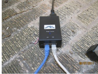
Illustration 5: LAN/POE Power Brick with both LAN and POE connected. LAN goes out to the Linksys Wireless G Router. POE goes out to the Rocket M5.
