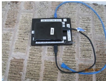
Illustration 6: Genesi SmartTop with 500 Gigabyte external hard drive on top. Ethernet cable (blue) is also shown.
