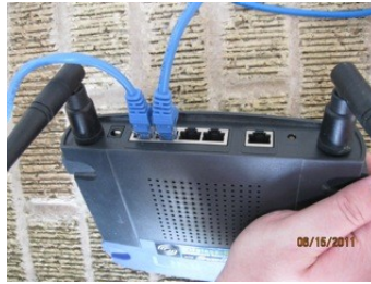
Illustration 8: The INTERNET Port is apart from Ports 1-4 and is clearly labeled INTERNET.
