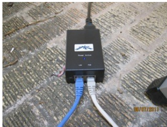
Illustration 6: LAN/POE power brick with both LAN and POE connected. LAN will connect to the Linksys Wireless G Router.
